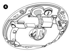
4. Feed the Ethernet cable from the bottom of the camera and through the hole. Attach the rubber seal plug for water proofing.
