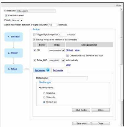
When completed the settings with steps 1~3 to arrange Schedule, Trigger, and Action of an event, click **Save event** to enable the settings and click **Close** to exit the page.
