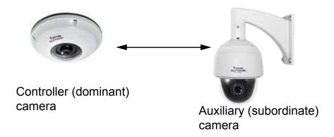
2. In a panoramic PTZ configuration, the fisheye camera provides an overview over the 360° hemispheric field of view; while the speed dome provides tracking, zooming, and keeping an object in a view of an adequate size. The configuration is operated via the VAST or Milestone software with easy clicks and drags.
