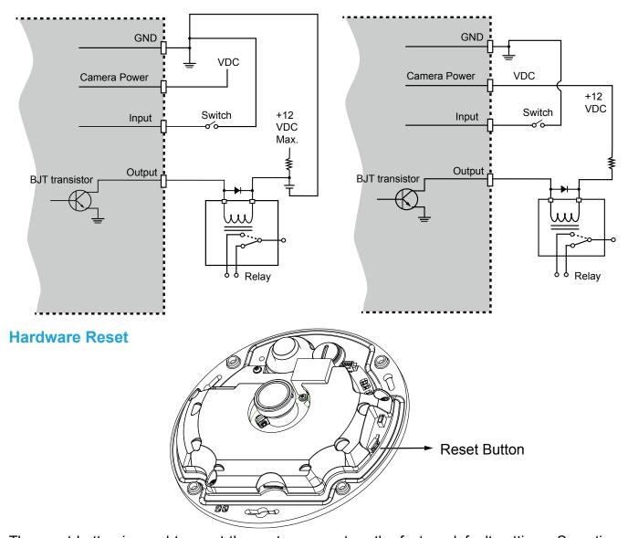
The reset button is used to reset the system or restore the factory default settings. Sometimes resetting the system can return the camera to normal operation. If the system problems remain after reset, press the reset button longer to restore the factory settings and install again.
