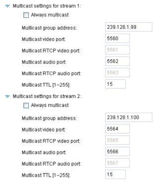
Unicast video transmission delivers a stream through point-to-point transmission; multicast, on the other hand, sends a stream to the multicast group address and allows multiple clients to acquire the stream at the same time by requesting a copy from the multicast group address. Therefore, enabling multicast can effectively save Internet bandwith.
