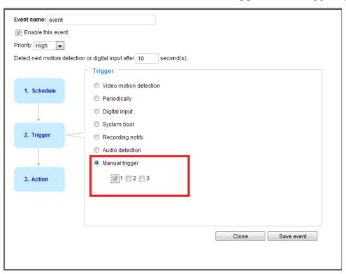
Note that the Manual trigger can last for another 10 seconds after the Controller (fisheye camera) returns to the normal state - no moving objects are detected.
