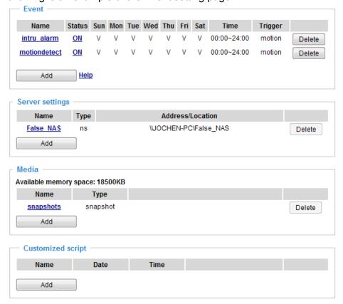
When the Event Status is **ON**, once an event is triggered by motion detection, the Network Camera will automatically send snapshots via e-mail.
