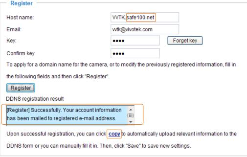
3. Click **Copy** and all the registered information will automatically be uploaded to the corresponding fields in the DDNS column at the top of the page as seen in the following screen.
