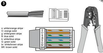
3. You will need an RJ45 crimping tool to attach the Ethernet wires to a connector. When done, connect the cable to the camera's Ethernet RJ45 socket.
