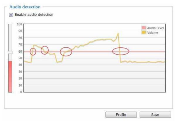
The red circles indicate where the audio alarms can be triggered when breaching or falling below the preset threshold.
