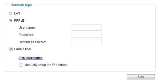
When IPv6 is enabled, by default, the network camera will listen to router advertisements and be assigned with a link-local IPv6 address accordingly.
