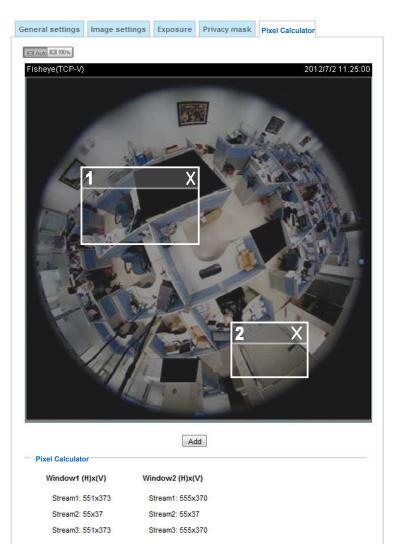
The pixels thus calculated are listed at the lower screen on a per-stream basis depending on the frame size you configure for each video stream.
